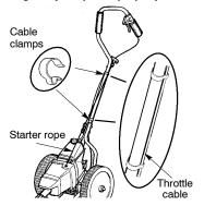
Align one cable clamp above the tube bolts and the other below the starter rope handle. Install the cable clamps one at a time around the tube and throttle cable.
