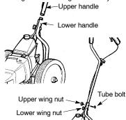
**NOTE:** When performing the following step, be sure the starter rope is not caught under the cable clamps. The starter rope must hang freely to operate properly.
