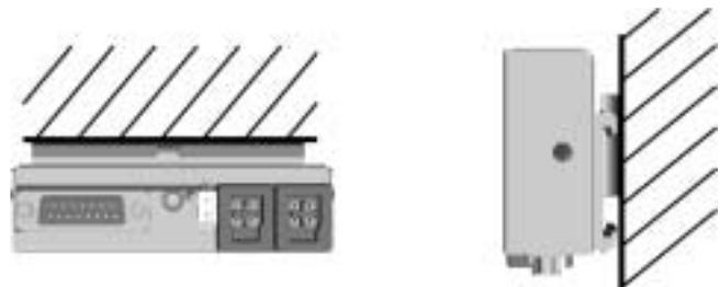
Parts supplied with the DX-ARC-SWB: Mounting bracket and screws
