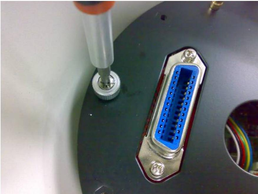
5. Loosen another screw (near the cradle). You can see the IP module.
