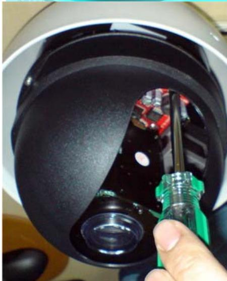
8. Follow anti-clockwise to fix the hemisphere cover onto speed dome.
