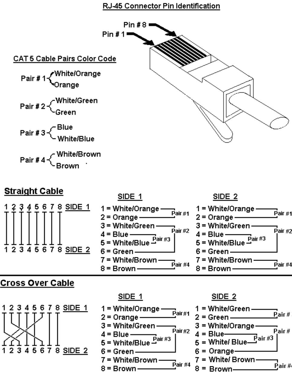
Figure 11: Cable Diagram
