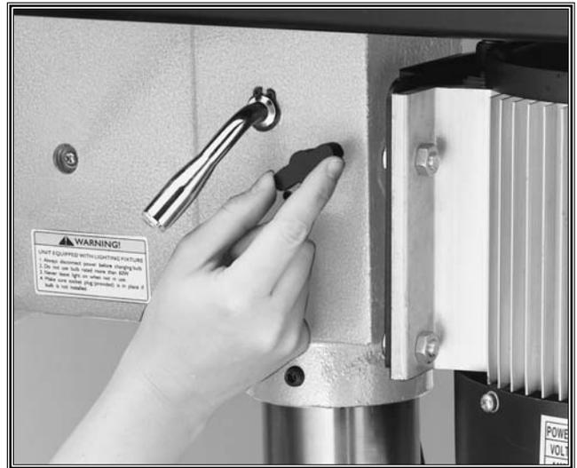
Figure 23. Loosening the lock knob.
