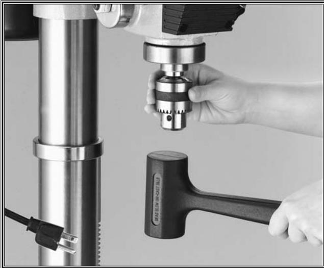
Figure 20. Seating arbor into spindle.
