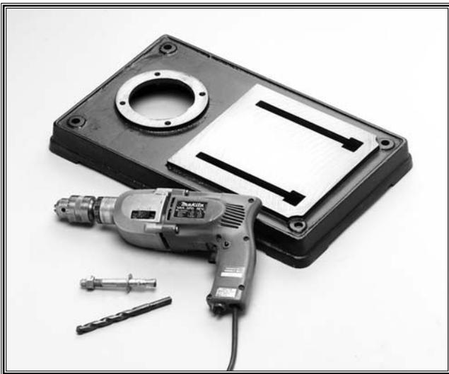
Figure 7. Secure base to floor.
