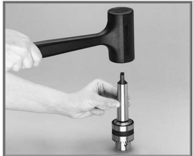
Figure 19. Seating the arbor into chuck.
