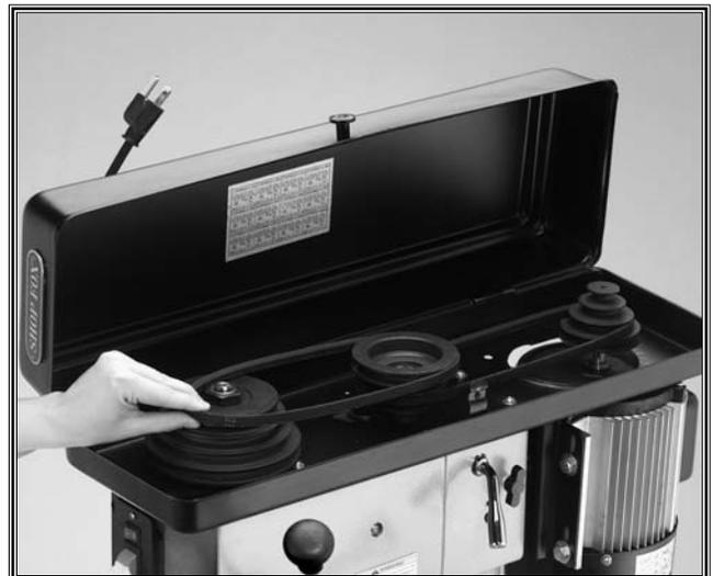
Figure 24. Adjusting belt to desired speed.
