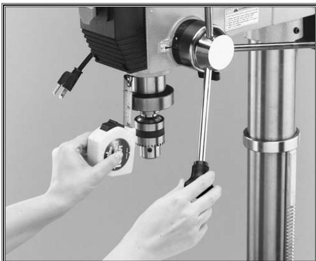
Figure 27. Actual stop depth being measured.
