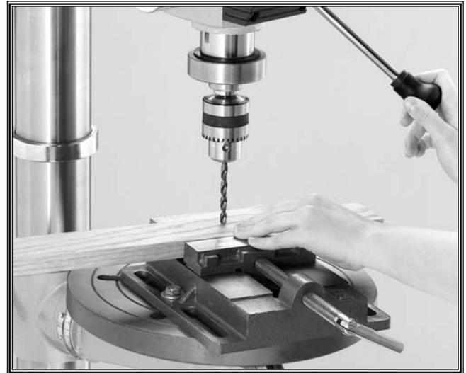
**Figure 3.** Keep fingers away from spinning tool.
