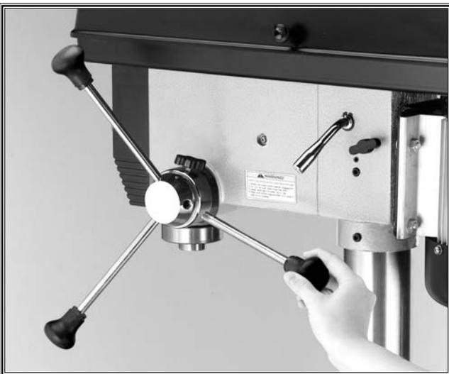
Figure 17. Installing handles.
