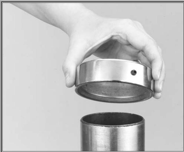
Figure 13. Inside bevel in the correct position.
