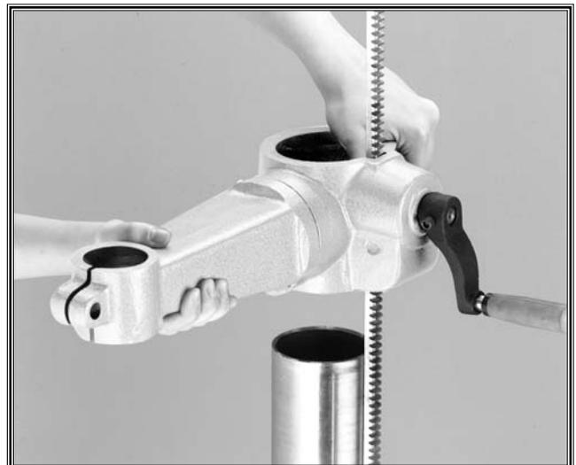
**Figure 11.** Correct rack orientation.
