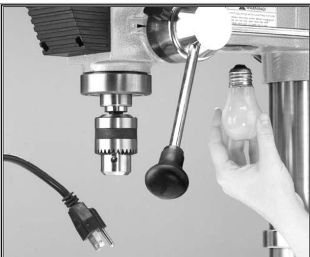
Figure 17b. Installing a light bulb.
