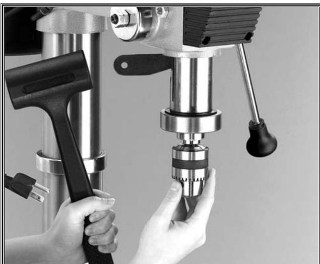
Figure 22. Using wedge to remove arbor.
