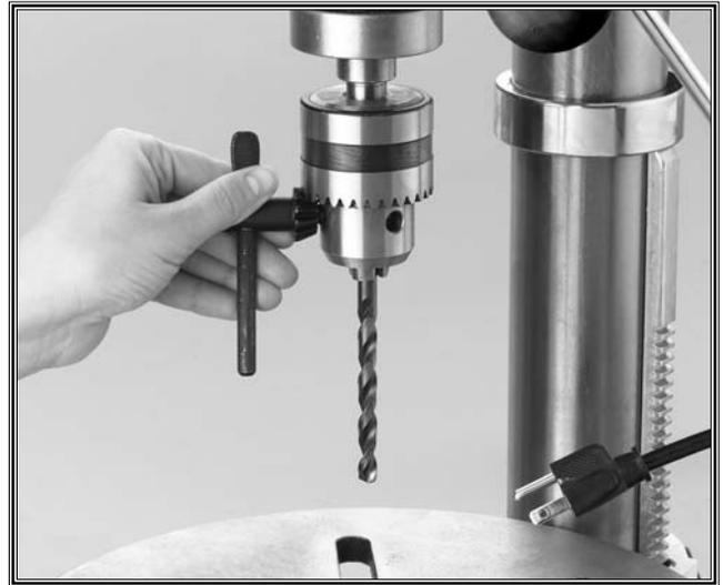
**Figure 33.** Chuck key engaged.
