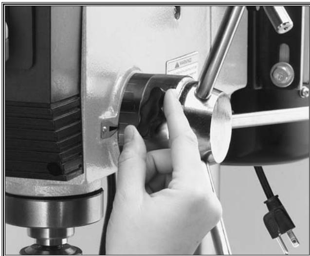
Figure 26. Loosening collar lock knob.
