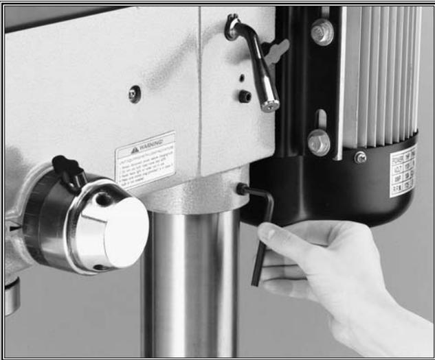
Figure 16. Tighten setscrews to secure headstock.
