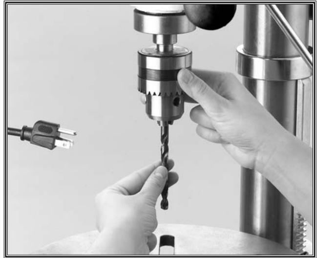
**Figure 32.** Installing bit.
