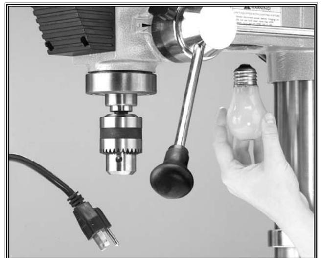
**Figure 5.** Unplug machine when changing bulbs.
