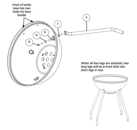
Do not tighten screws all the way. Legs may need to be adjusted when storage shelf is attached in STEP 3.
