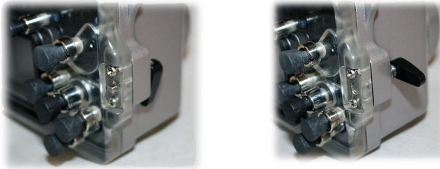
Pull out the lid by holding on the grip near the lock.
