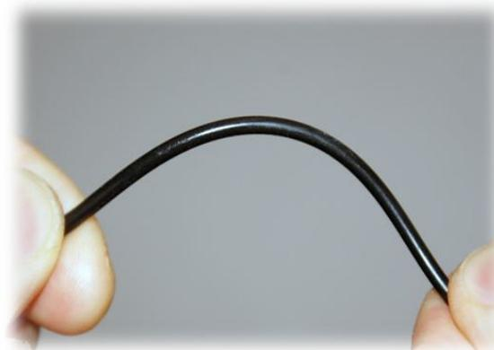
Once the O-ring has been inspected and verified fit for use, apply a small amount of silicone grease to the O-ring. The silicone grease must be evenly distributed round the O-ring. Install the O-ring into the groove; run a finger round the O-ring, to make sure it is snugly seated in the groove.
