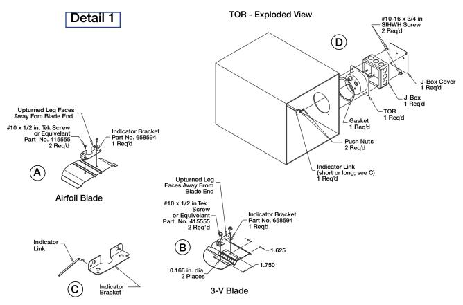
Note: Indicator Link Part Nos For Standard Sleeve (short): 457808 For Extended Sleeve (long): 457801 Note: Operator Mounted Upside-Down On Steel Airfoil Units From 10 in. to 17 in. (254mm to 432mm) High
