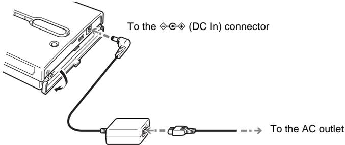
When the AC power adapter is connected to the unit, the internal battery starts charging. The
