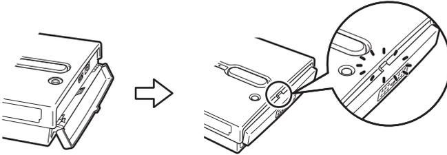
To solve this problem, press the center of the cover as illustrated until it is in its fully open position, and then try closing it again.
