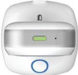
The indicator LED will glow **green** and flash on and off. After a few seconds, the LED steadily glows green. This means the camera is ready for remote connection.
