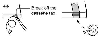
If you later want to reuse the tape for recording, cover the broken tab with adhesive tape.
