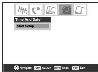
If you have not set up the TV Guide On Screen™ system, the following screen will appear. To set the time, highlight **TV Guide On Screen™** and press **ENTER**. The TV Guide On Screen™ setup sequence will start, and the time and date will be set automatically.
