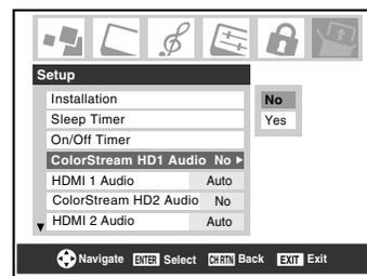
**Note:** The analog audio terminals for the ColorStream HD and HDMI inputs are used in common. When the ColorStream HD 1 (or 2) audio mode is set to **Yes**, the HDMI 1 (or 2) audio mode is set to **Digital** and will be grayed out. When the ColorStream HD 1 (or 2) audio mode is set to **No**, the HDMI 1 (or 2) Audio changes to **Auto**.
