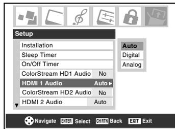
**Note:** The ColorStream HD1/HD2 Audio settings influence the HDMI Audio settings. If ColorStream HD1 (or 2) Audio is set to **No**, the HDMI 1 (or 2) Audio setting changes to **Auto**. If either ColorStream HD1 (or 2) Audio is set to **Yes**, the HDMI 1 (or 2) Audio setting is set to **Digital** and will be grayed out.
