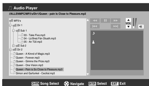
To expand a particular folder to view a list of images, press **▶** on the folder. To close the folder or directory, press **◀** on the folder or directory. Pressing **◀** on a file will move the focus up to the folder which contains the file. Pressing **▶** on a file will move the focus down to the next folder.
