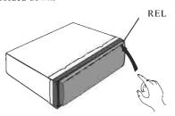
When the front panel was turned down to a position of 45°, hold and slide the front panel to left, and then pull it out.
