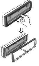
2.Insert the keys supplied to the unit at both sides of the unit (shown as illustrated) until they click. Pulling the keys makes it possible to remove the unit from the dashboard.
