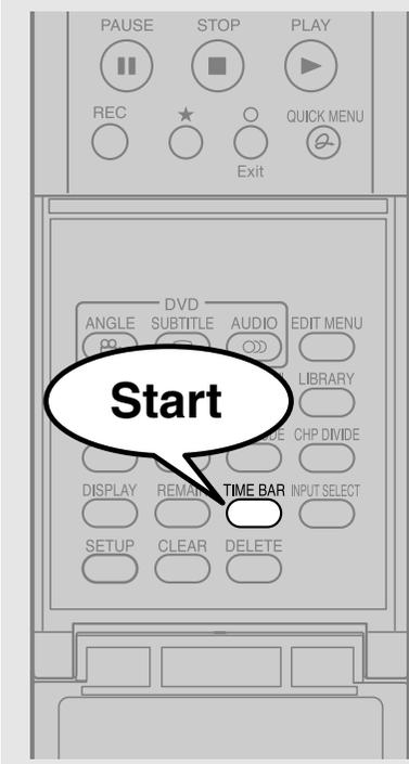
**1 During playback or recording, press TIME BAR.**
