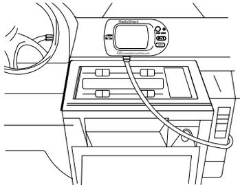
**Note:** When you choose a mounting area for the controller, make sure it is close enough to the Audio Adapter's mounting area so the controller's cord will reach the Audio Adapter. The controller's cord is about 5 feet (152 cm) long.
