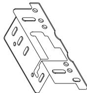
3. Using the supplied mounting studs as templates and the width between the mounting brackets as a guide, mark the positions for the mounting holes.
