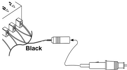
4. Connect the Audio Adapter's red power wire (with inline fuse holder) to a point in your vehicle's fuse block that has power only when you turn the vehicle's key to either the accessory (ACC) or START position.
