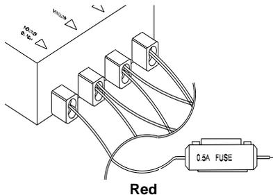
This connection turns on the CD changer and its components when you turn on the ignition or turn the key to ACC, and turns off the CD changer and its components when you turn off the ignition. This prevents your vehicle's battery from being drained if you leave the CD changer on when you turn off the ignition.
