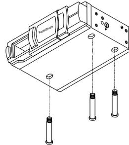
Save the shipping screws in case you might want to install the CD changer in another vehicle. You can secure them to the back of the CD changer with a piece of tape.
