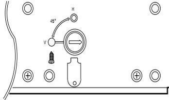
**Caution:** If you do not set **SPRING ATTACHMENT H/V** on both sides of the CD changer to the correct mounting axis, the CD changer might skip during play.
