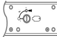
If you are mounting the CD changer vertically, use a screwdriver to remove the screws on both sides of the CD changer from **H** and turn **SPRING ATTACHMENT H/V** to **V** on both sides, then replace the screws into **V**.
