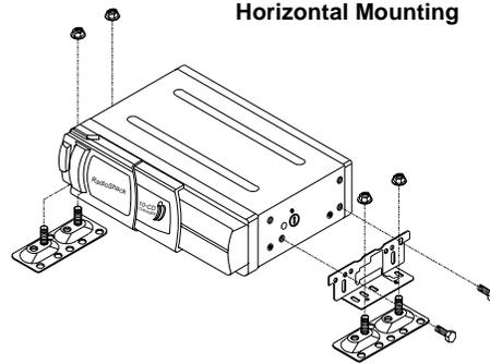
1. Set **SPRING ATTACHMENT H/V** (horizontal/vertical) on both sides of the CD changer for the mounting axis you chose.
