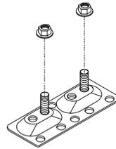
5. Attach the CD changer to the mounting studs using the supplied nuts.
