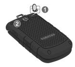
2. Use the grooves at the top of the cover to lift the cover up and away from the back of the phone (1).
