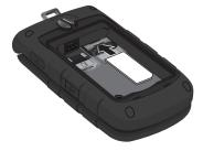
To remove the SIM, gently slide it out of the socket.
