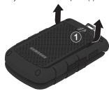
Lift the battery up (1) and away (2) from the phone, as shown.
