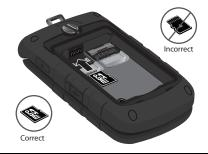
Warning!: Please note the printed circuit side faces down when inserting the card.
