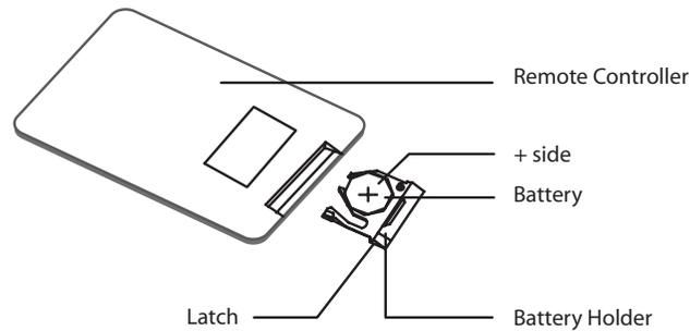
1. Move the small latch to the right and slide out the battery holder.
