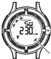
NOTE: If there is no key manipulation for 20 seconds, the compass sensor will be deactivated for power saving and the watch will display only the current HOME TIME or FOREIGN TIME (depends on your selection in time mode). Press S1 button to re-activate the compass sensor.
