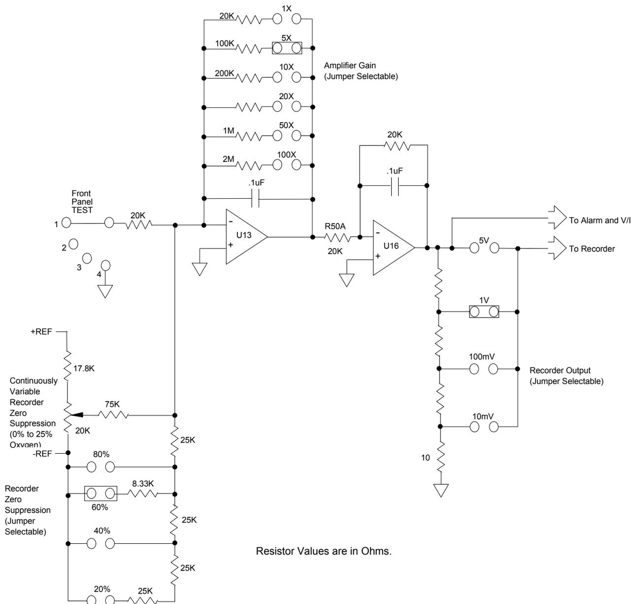
Figure 5-10. Simplified Analog Output Circuit for Recorder (Showing Three Ranges)
