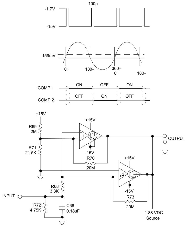
Figure 5-1. Two-Comparator OR Circuit
