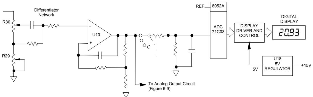
**Figure 5-9. Buffer, Anticipation, and Digital Output Circuit**
