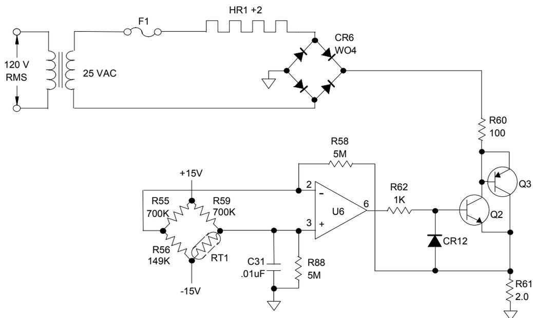
**Figure 5-5. Detector Heater Control Circuit**
