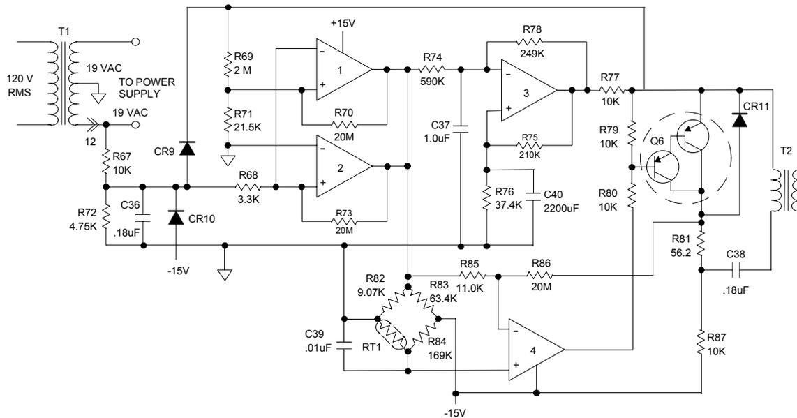
Figure 5-3. Case Heater Control Circuit
