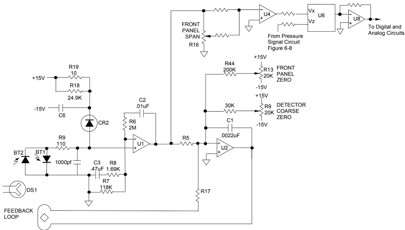
Figure 5-7. Detector with First Stage Amplifier and Pressure Compensation Circuits
