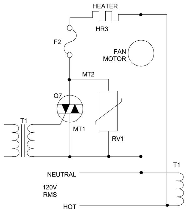
**Figure 5-4. Case Heater Circuit**
