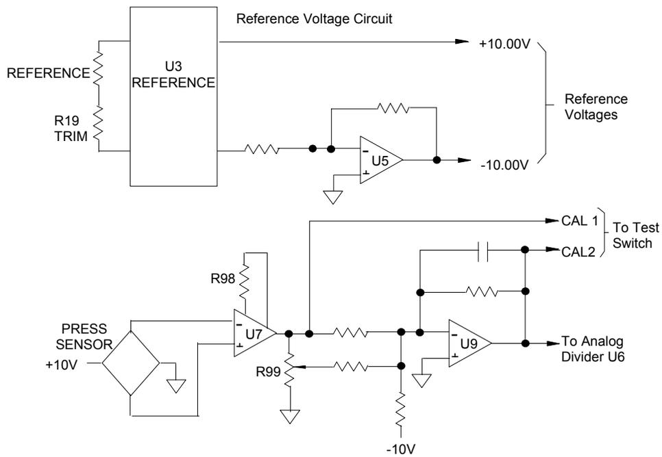
Figure 5-8. Pressure Signal and Reference Voltage Circuits
