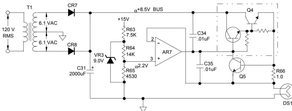
Figure 5-6. Detector Light Source Control Circuit
