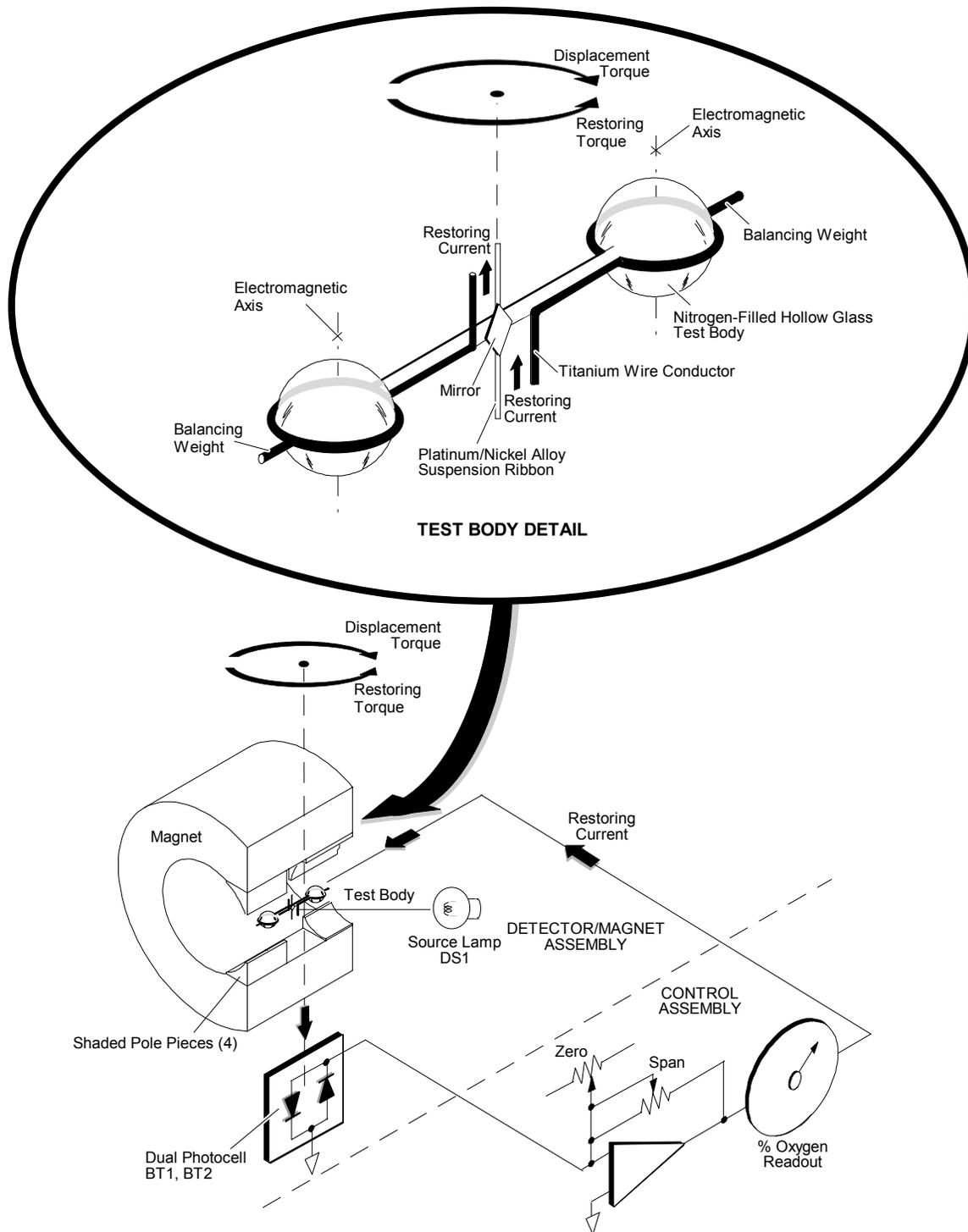
Figure 4-2. Functional Diagram of Model 755A Paramagnetic Oxygen Measurement System
