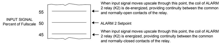
Figure 2-5. Typical Alarm Settings
