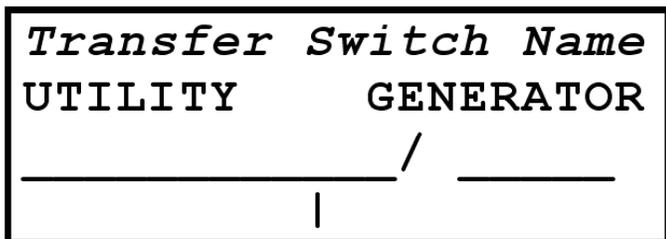
This is the Transfer Switch Mimic Diagram page. It shows the position of the Utility Switch and the Generator Switch. This depicted display shows the Utility switch closed and the Generator switch open. There can be up to 4 HTS switches connected to the generator.
