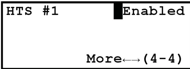
For this example, HTS number 1 is now enabled. If HTS #1 is not connected or if the HTS is not #1, there will be a communications error indicated.
