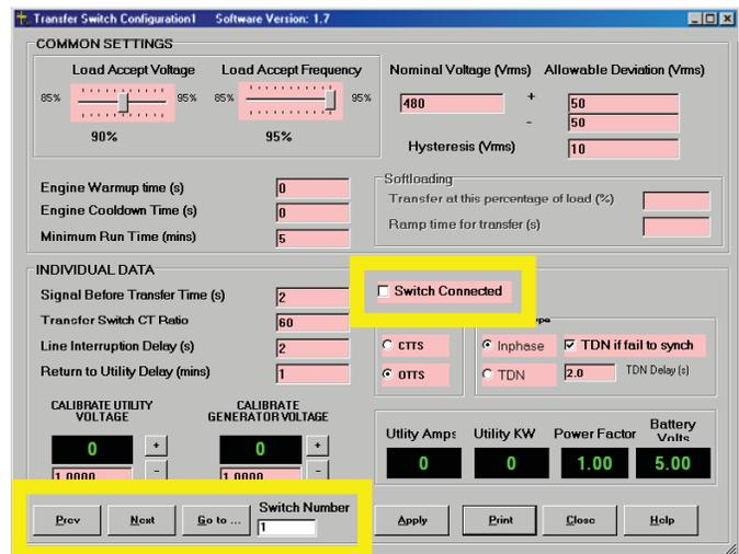
The lower left corner contains the HTS number. Use the “Prev” and “Next” buttons to select the appropriate switch number - 1 through 4. If enabling the switch, check the “Switch Connected” check box in the middle of the screen. If disabling the switch, uncheck the “Switch Connected” check box. The remainder of the settings on this page are described in the HTS manual.
