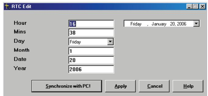
Any of the fields are editable. Note that hours are entered as 0 – 23. If the PC being used has reliable date and time settings, pressing the “Synchronize with PC!” button will copy the PC date and time into the H-100 Control Panel. Otherwise, press “Apply” after making changes. The date and time on the GenLink screen may take a few seconds to update.
