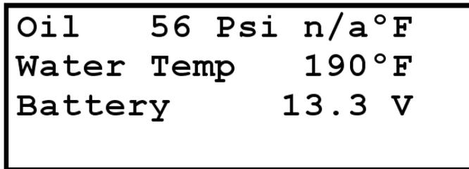
This is a typical Home page. The contents of this page along with the contents of the default left display page (Volts) were selected such that all the normally desired data would be available for viewing at once.
