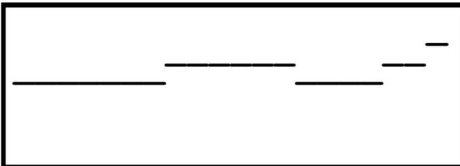
This is the Generator Frequency Graph page. This graph provides a coarse representation of the generator frequency. The graph scrolls from right to left at 2 characters per second (last 10 seconds of data on the display). The bottom of the graph is 50 Hz and the top is 70 Hz. There are 32 levels between bottom and top. Therefore, each level is approximately 0.6 Hz.
