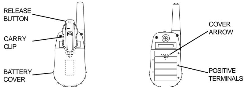
1. Using thumb, press down on battery cover at arrow and slide cover down to open.
