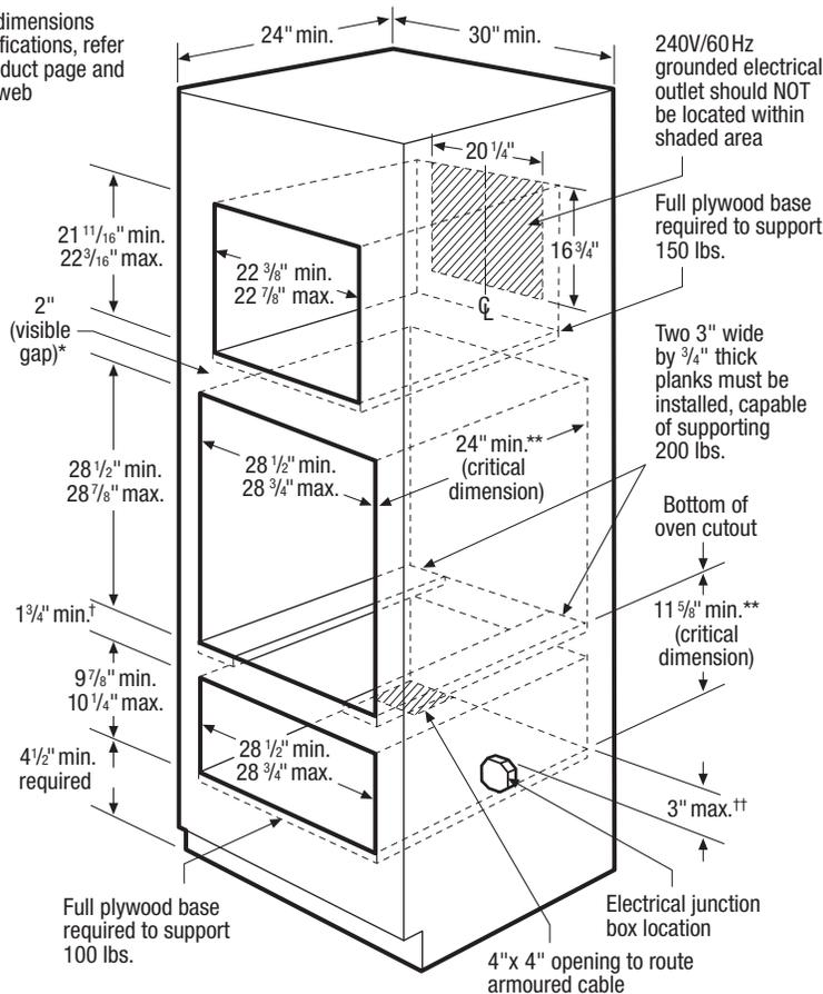
\* Minimum 2<sup>5</sup>/<sub>8</sub>" clearance required from bottom of Built-In High-Speed Oven cutout to top edge of Wall Oven's faceplate, leaving a 2" visible gap between both product faceplates
