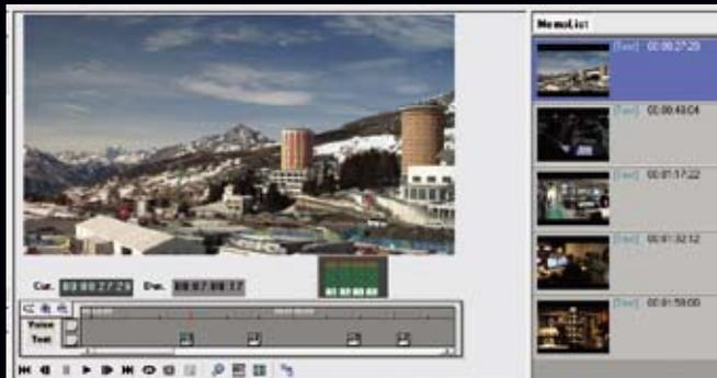
This shows the text memo editing window of the provided Windows PC software, P2 Viewer. A list of memos is shown on the right side. The clip time line below the view window shows the memo marks. Text can be written to an empty memo space created by the camera-recorder. Memos can also be added, deleted or moved.
