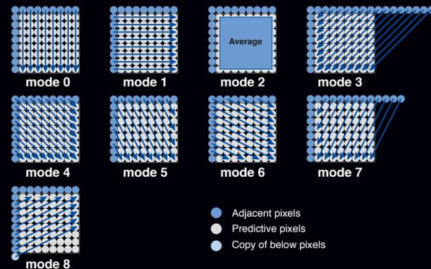
This process generates predictive images based on adjacent blocks of 8 x 8 pixels. Selecting the most suitable predictive mode from among nine luminance signal modes (see illustration) and four color signal modes, it generates accurate predictive images.
