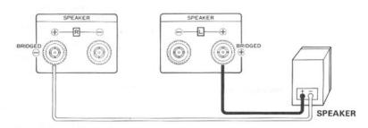
Strip 1.0cm (3/8") of the polyvinyl chloride insulation from the end of each speaker lead. Twist the exposed strands tightly, and secure the end with a touch of solder.
