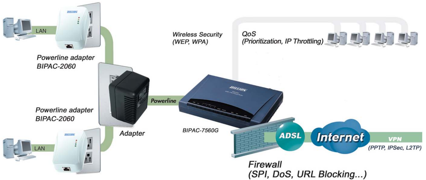
Figure 1.1 Application Diagram of BIPAC-7560 Powerline ADSL VPN Firewall Router
