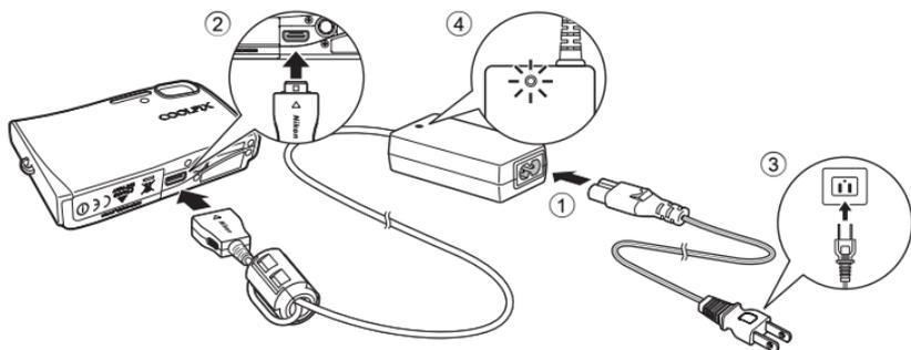
**1** Connect the power cable and AC adapter ①.
