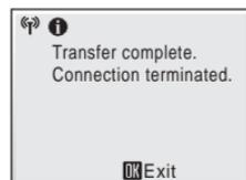
\* Once upload of all pictures, which is initiated by connecting the AC adapter, is complete, the camera turns off and the battery begins charging.
