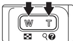
When the camera is zoomed in to the maximum magnification (3 $\times$ ), holding down **T** (🔍) triggers digital zoom. The subject is magnified up to 4 $\times$ , for a total magnification of 12 $\times$ .
