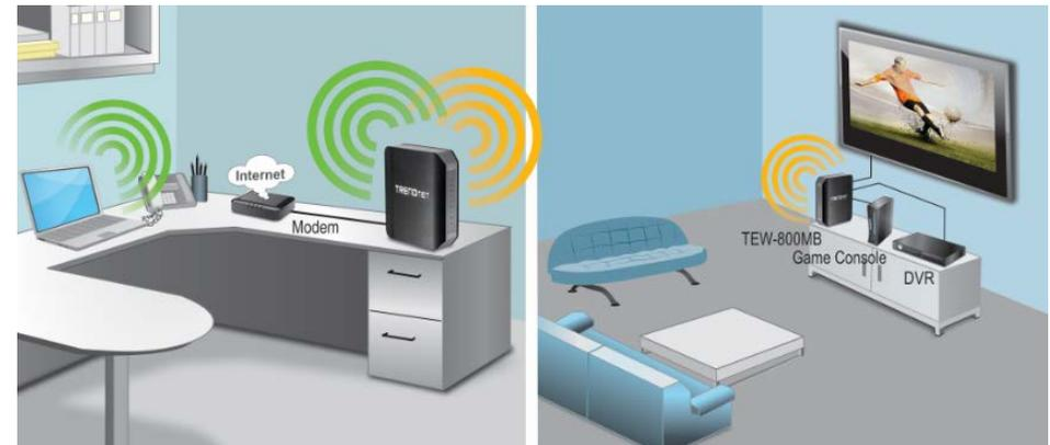
The router's gigabit Internet port is connected to your Internet modem which is connected to the Internet. Wireless signals from the router are broadcasted to wireless clients such as laptops (with wireless capability), TVs or media bridges thereby providing Internet access.
