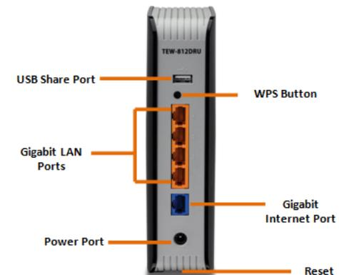
4. Using a Network cable, connect the gigabit Internet port on the router to your modem.
