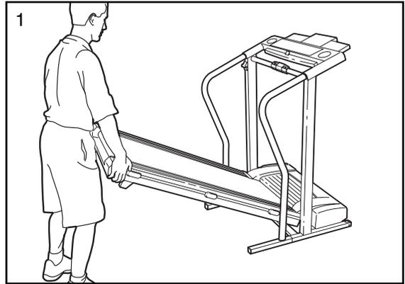
2. Move your right hand to the position shown and hold the treadmill firmly. Hold the lock knob with your left hand and pull it to the left. Raise the treadmill until the lock knob is aligned with the slot in the catch. Note: You may need to push the handrail to the side slightly. Slowly release the lock knob. **Make sure that the pin on the lock knob is inserted into the slot.**
