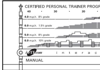
The profiles on the console show how the speed and incline of the treadmill will change during the personal trainer programs. The numbers beside the profiles show the maximum speed and incline settings for the programs. For example, the upper profile shows that the treadmill will reach a maximum speed of 4.0 mph and a maximum incline of 8% during the first program. The TIME/INCLINE/MIN-MILE display will show how long the selected program will last.
