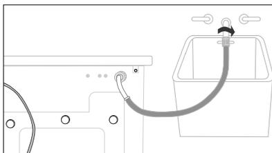
2. Connect the other end of the cold water supply hose to your sink's cold water faucet and tighten it by hand. If necessary, you can reposition the water supply hose at the washing machine end by loosening the fitting, rotating the hose, and retightening the fitting.
