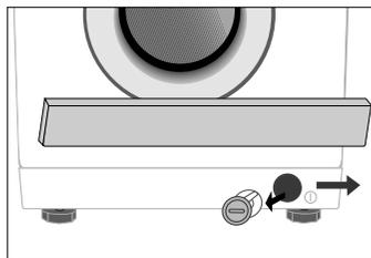
4. Wash any dirt or other material from the filter. Make sure the drain pump propeller behind the filter is not blocked. Replace the filter cap.
