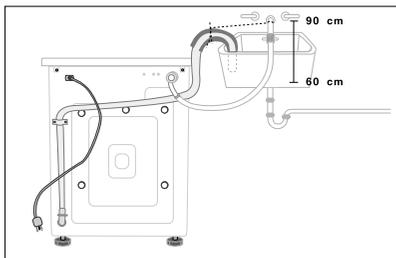
In a sink drain pipe branch
