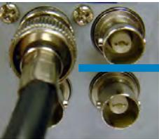
Push and twist the BNC connector clockwise to secure it to the BNC port.
