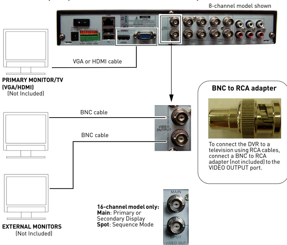
On the 16-channel model, connect external monitors to either the **Main** or **Spot** port.
