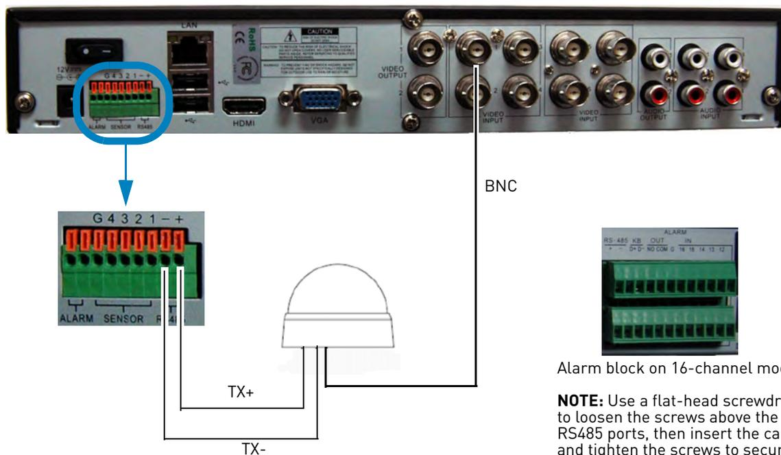
Alarm block on 16-channel model
