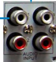
Connect an RCA audio cable from the camera into the corresponding Audio INPUT port
