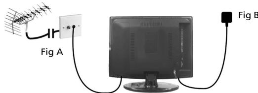
3) Switch on the television using the power on/off switch located on the rear of the TV.
