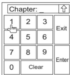
Enter the desired chapter/track using the on-screen number pad. Press the **Enter** button to tune to the selected station. To exit the screen without changing the station, touch **Exit**. To clear your entry and start over, touch **Clear**.
