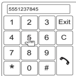
2. Use the 0-9, \*, and # buttons to input the phone number. Touch the **C** button to clear the last digit.
