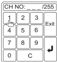
Enter the desired radio station using the on-screen number pad. Touch the arrow (enter) button to tune to the selected station. To exit the screen without changing the station, touch **Exit**. To clear your entry and start over, touch **C**.
