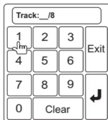
Enter the desired track using the on-screen number pad. Press the enter button (arrow) to play the selected track. To exit the screen without selecting a track, touch **Exit**. To clear your entry and start over, touch **Clear**.
