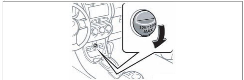
Designed for car accessories. Key must be in the “ACC” or “ON” position for use.
