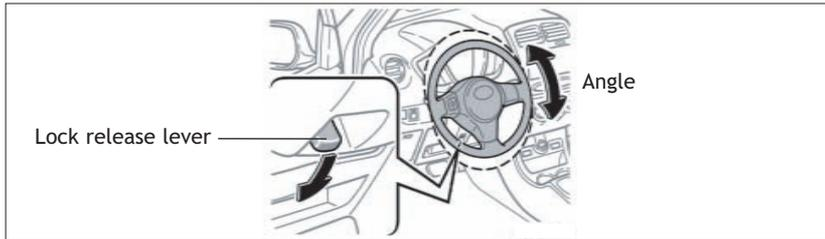
Hold wheel, push lever down, set angle and return lever.
