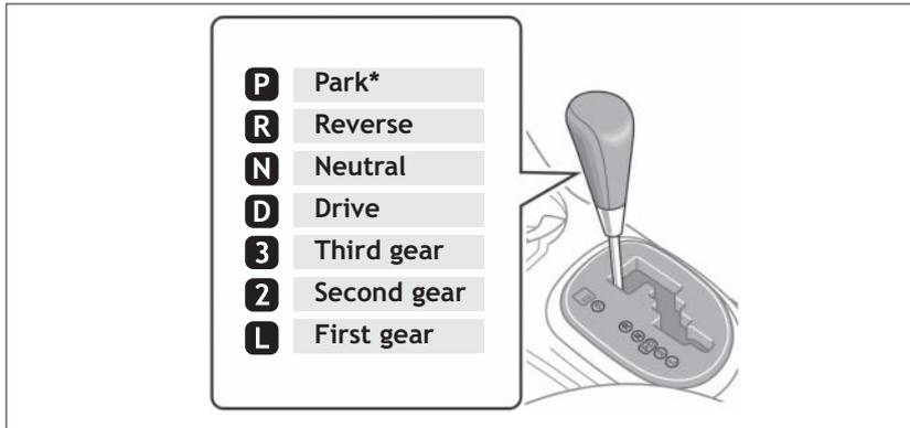
\* The engine switch must be "ON" and the brake pedal depressed to shift from Park.
