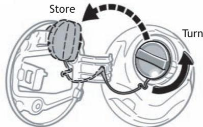
**NOTE:** Tighten until one click is heard. If the cap is not tightened enough, Check Engine indicator may illuminate.
