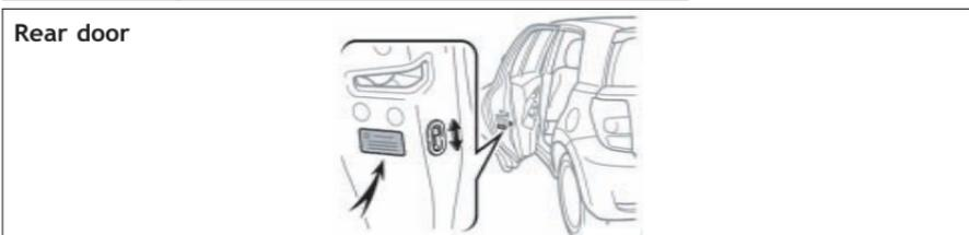
Moving the lever to "LOCK" will allow the door to be opened only from the outside.
