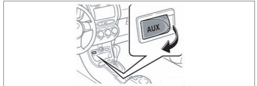
By inserting a mini plug (not included) into the AUX jack, you can listen to music from a portable audio device through the vehicle’s speaker system while in AUX mode.
