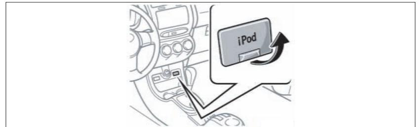
By inserting the standard iPod® connector cable into the iPod® jack, you can charge the iPod® battery, control the iPod® functions using the car audio unit and listen to music from your iPod® through the vehicle’s speaker system.
