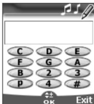
To select a note, press on the corresponding key on the keypad (regardless of the letters on the keypad).
