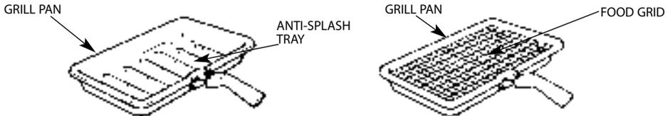
**Note:** To stop fat splashing onto the grill mesh, it is important to use the anti-splash tray as shown in the grilling chart. Always clean the grill pan, anti-splash tray and food grid after each use.
