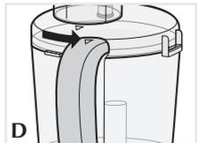
3. Place food chute/cover onto container with food tube to the left of the handle. Twist food chute/cover counterclockwise until you hear it click into place and LOCK. Arrow on handle aligns with arrow on the chute/cover (D).
