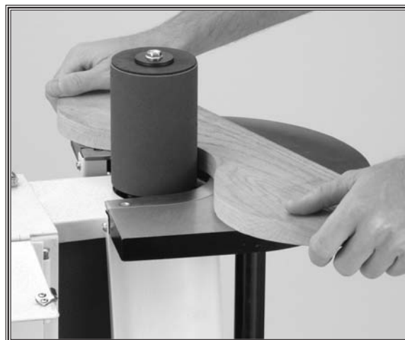
Figure 30. A typical spindle sanding operation.
