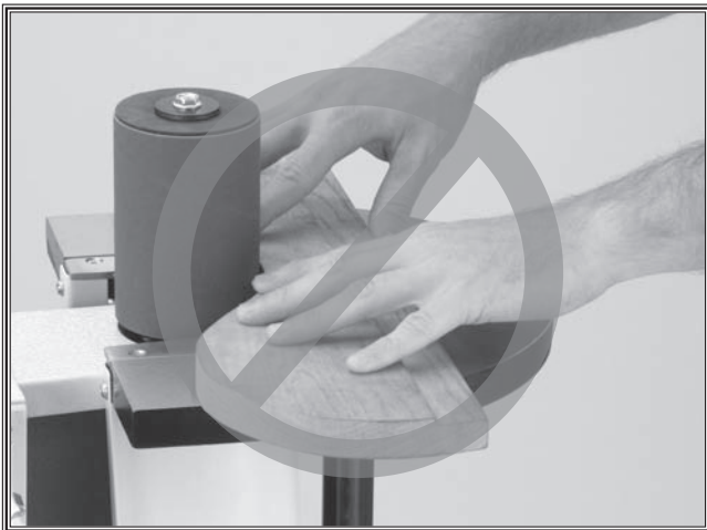
Figure 3. DO NOT sand wood with fingers close to spindle.
