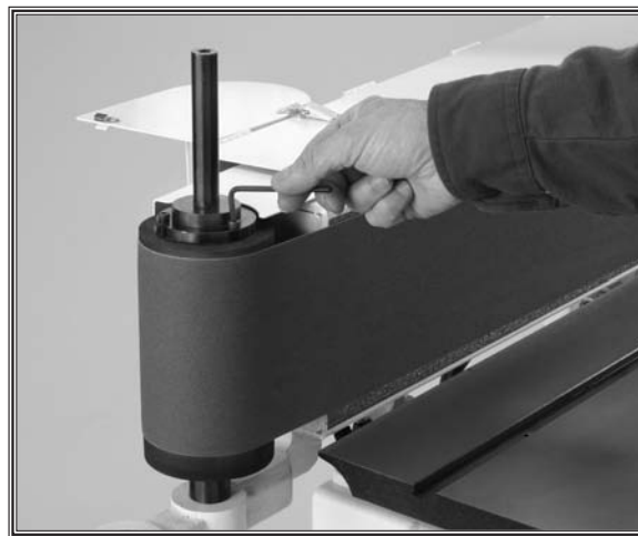
Figure 17. Securing the cap screws.
