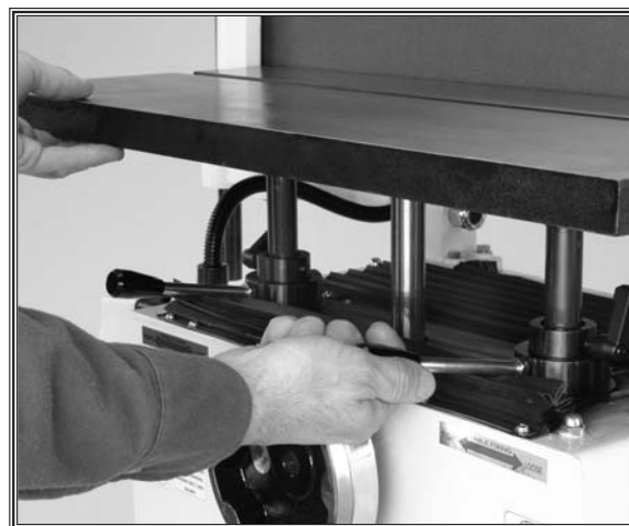
Figure 26. Horizontal table adjustment.
