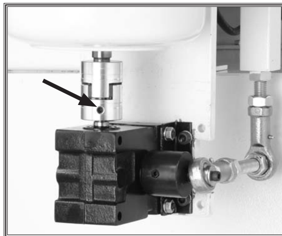
Figure 35. Spindle connector set screws.
