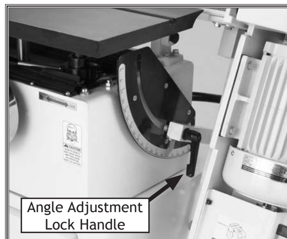
Figure 24. Platen angle scale.
