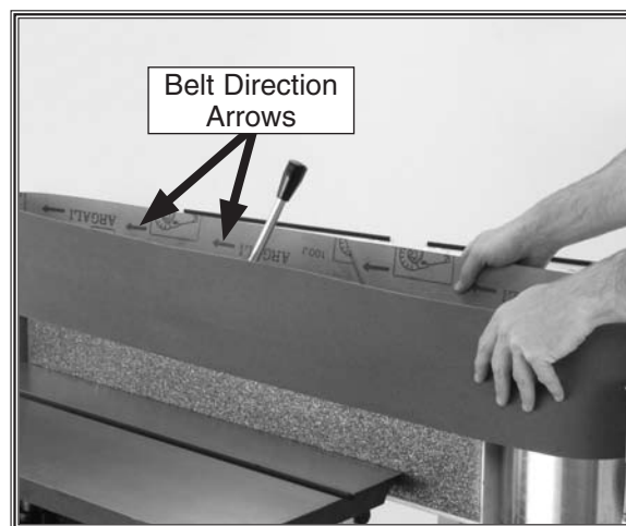
Figure 12. Placing the sanding belt onto the sanding drums.
