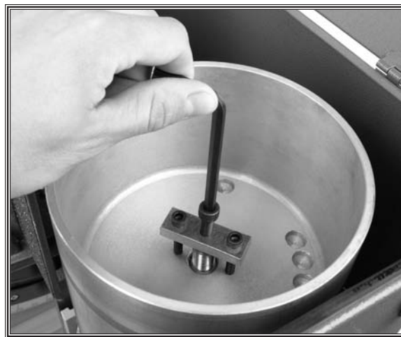
Figure 39. Using the drive roller puller.
