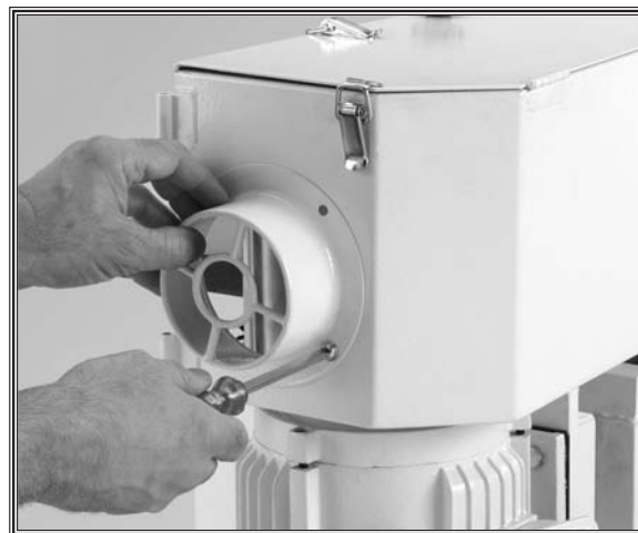
Figure 14. Dust port installation.
