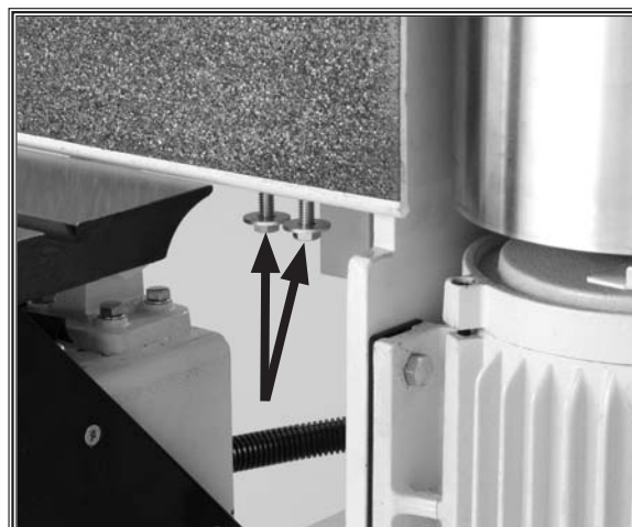
Figure 13. Backstop bolts threaded into platen.
