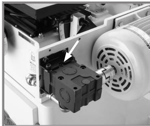
Figure 32. Gear box and oil fill on the Model W1730.
