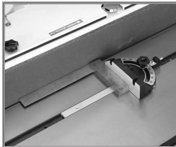
Figure 27. Squaring the miter gauge.
