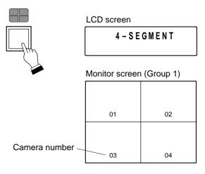
Step 2. Press the 4-Segment Split-Screen key again, or the Group Selector key. The images of camera numbers 5 – 8 (Group 2) will be displayed on the monitor.
