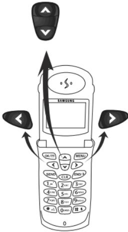
**3. Navigation Keys:** These keys allow you to scroll when viewing menus, the phonebook, browser, etc., and to move the cursor when editing any option. Also, each navigation key has a one-touch special function that it performs. Here are the one-touch special functions:
