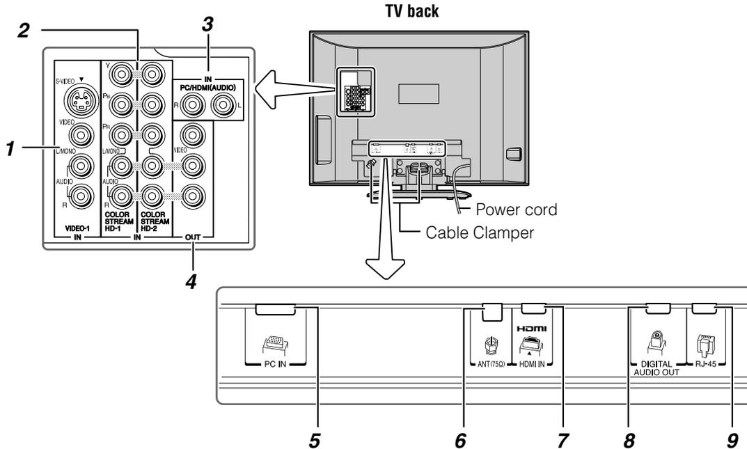
**1 VIDEO-1 IN** — Standard (composite) video and standard audio inputs plus optional S-video inputs for connecting devices with composite video or S-video output.
