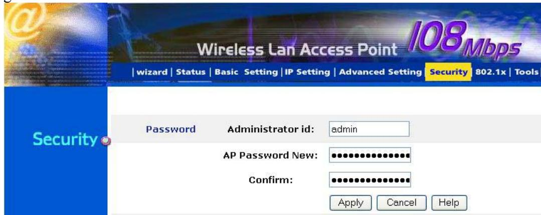
The screenshot shows the configuration interface for a Wireless LAN Access Point. The main heading is "Wireless Lan Access Point 108Mbps". Below the heading is a navigation bar with links: "wizard | Status | Basic Setting | IP Setting | Advanced Setting | Security | 802.1x | Tools". The "Security" link is highlighted. On the left side, there is a blue sidebar with the word "Security" and a small icon. The main content area is titled "Password" and contains the following fields and buttons:
