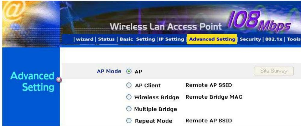
**1 AP:** The normal Access Point operating mode which forms a wireless ESS network with its wireless clients. In figure an example of configuration.
