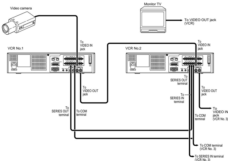
The SERIES OUT signal will be present either at the point when the counter reading is 7H57M00S or when VCR No. 1 reaches the end of the tape, whichever is first. The signal will stop 70 seconds after the tape end point of VCR No. 1.
