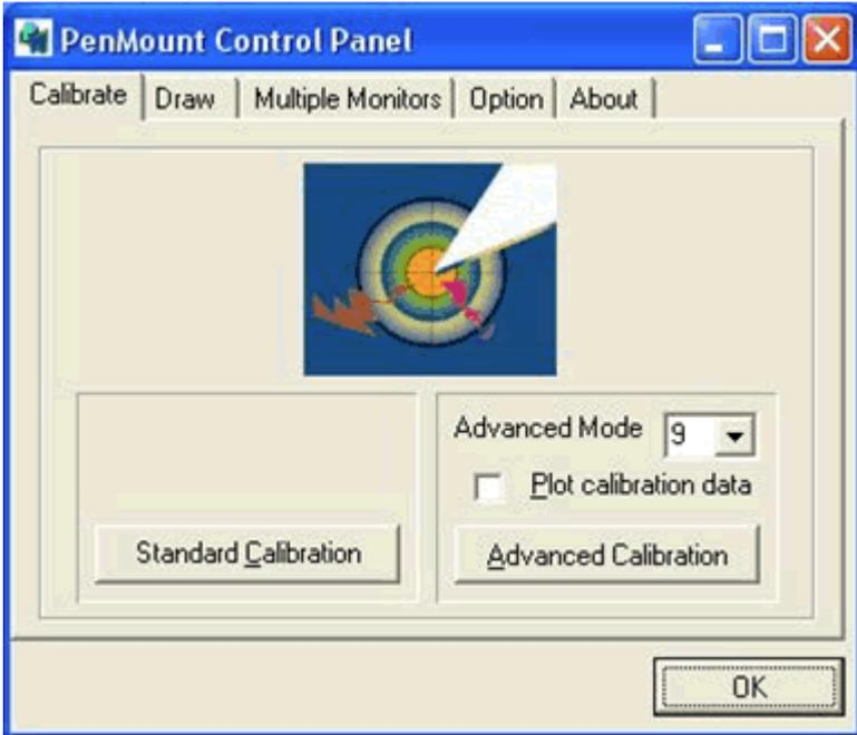
*NOTE: The older the touch screen, the more Advanced Mode calibration points you need for an accurate calibration. Use a stylus during Advanced Calibration for greater accuracy.*
