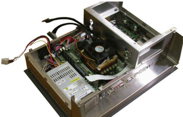
6. Push the two white eject levers on each side of the DIMM outward until they are separated from the black vertical posts.
