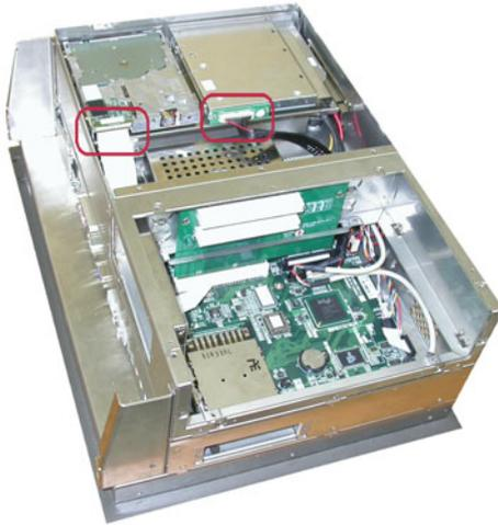
3. Unscrew the screws of the FDD and CD-ROM module and take off the FDD and CD-ROM.
