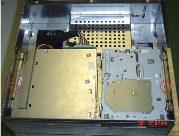
3. Remove four screws and take off HDD bracket.
