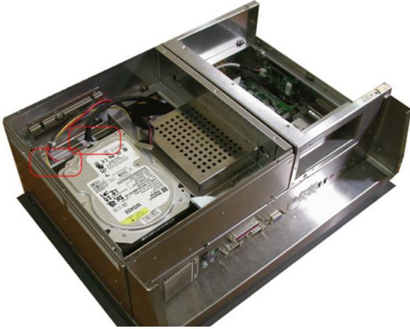
5. Undo the seven screws of the HDD Module so you can install the SDRAM.
