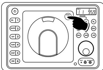
2. Insert the disc onto the hub with the label facing forward. Use your thumb to make sure the disc snaps onto the hub.
