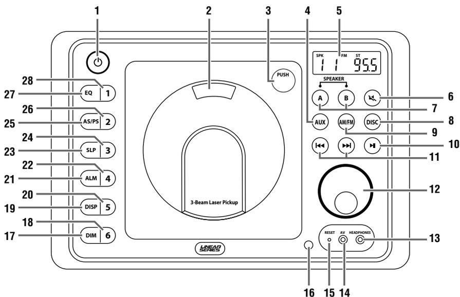
1. **Power On/Off:** Press to turn the unit on or off.
