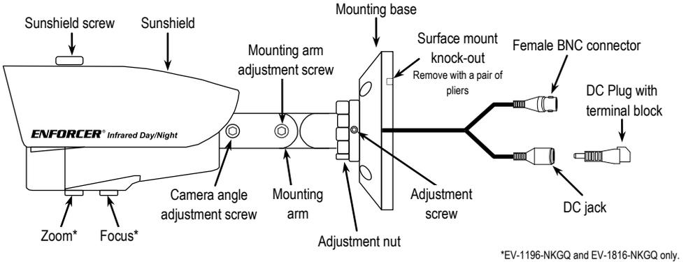
ENFORCER IR LED Bullet Cameras can be mounted to a standard lamp holder cover plate (not included).
