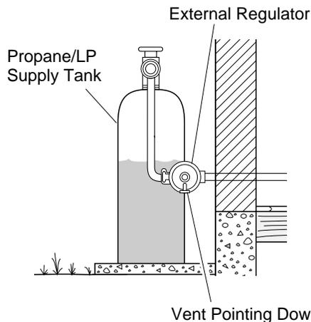
Figure 22 - External Regulator with Vent Pointing Down
