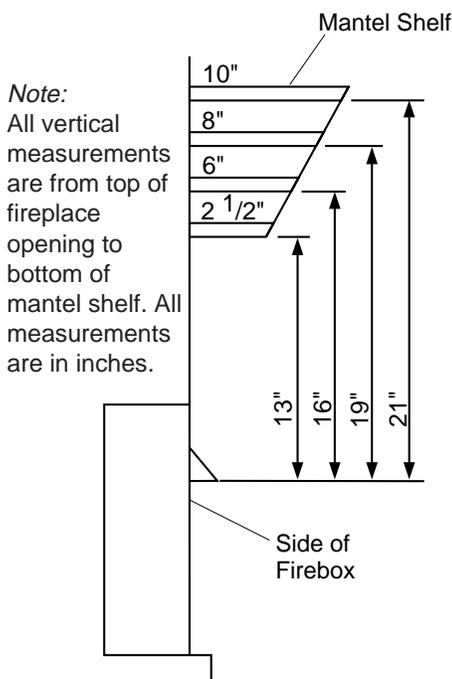
**Figure 11 - Minimum Mantel Clearances for Built-In Installation**
