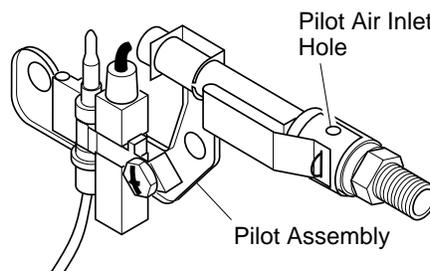
**Figure 36 - Pilot Inlet Air Hole**
