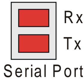
Figure 3.4 – Automation Equipment Port Receive & Transmit LEDs The LED's flash when the TIU10X is communicating with the AE.
