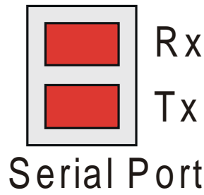
Figure 4.4 – Automation Equipment Port Receive & Transmit LEDs
