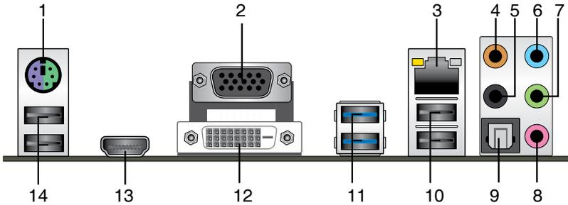
1. **PS/2 keyboard/mouse combo port.** This port is for a PS/2 keyboard or mouse.
