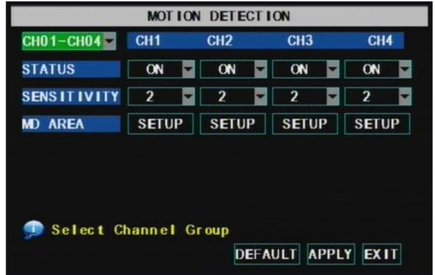
Next, click on the MD AREA SETUP button, which will display the picture on the left. This option allows you to select the area you want to be sensitive to motion. The area in red is sensitive to motion. You can set this area by using the mouse or REV, FWD, and SEL keys on the front panel. Once you have set the area, right click with the mouse or push the ESC key to save the setting. After you have set all of the cameras, click on the Apply button to save the settings.
