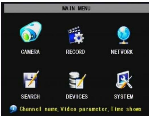
Choose MENU by right clicking on the mouse or by pushing the MENU button on the DVR front panel or remote control.
