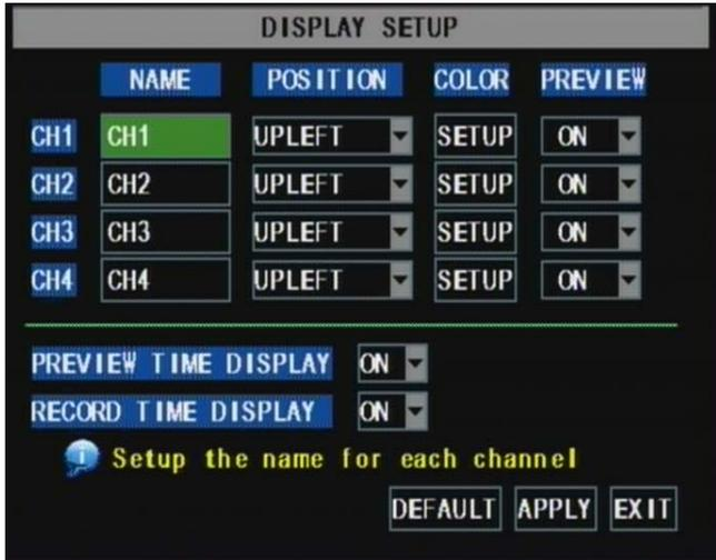
From the Main menu, select CAMERA. Here you can setup the name display (up to 8 characters) and position of each channel (cameras). Select COLOR SETUP to adjust the image brightness, saturation, contrast and hue settings for each channel (camera). You can also choose whether each channel can be previewed in LIVE MODE and/or RECORDING MODE.
