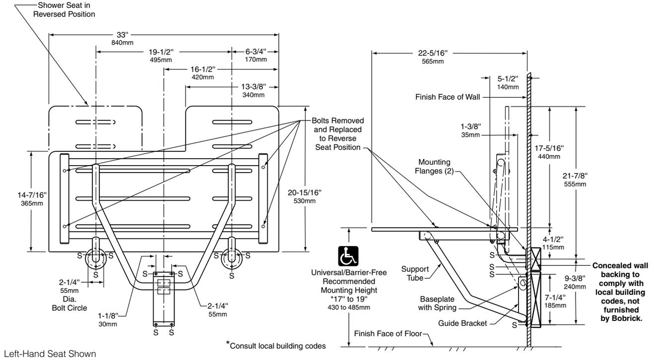
**Installation to Wall.** Secure unit to wall at points indicated by an S, with the two Mounting Flanges located at top and the Baseplate and Guide Bracket below. The bottom of the Support Tube must be positioned within the Baseplate and Guide Bracket before they are secured to wall. \* Mounting height of shower seat must comply with local building codes.
